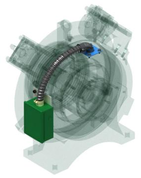
Figure 24: Factory Side Mount Electrical Box Relocation Example. Field Kit Available
