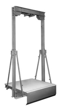
At Hollister-Whitney we supply you with a complete line of passenger and freight car slings and platforms for both hydraulic and traction installations. Each car sling and platform assembly is supplied complete with channel stiles, crossheads, gussetts, braces, cable hitch plates (traction jobs only), cutout for sills, #26GA fireproofing on underside of wood platform, and one toe guard.
