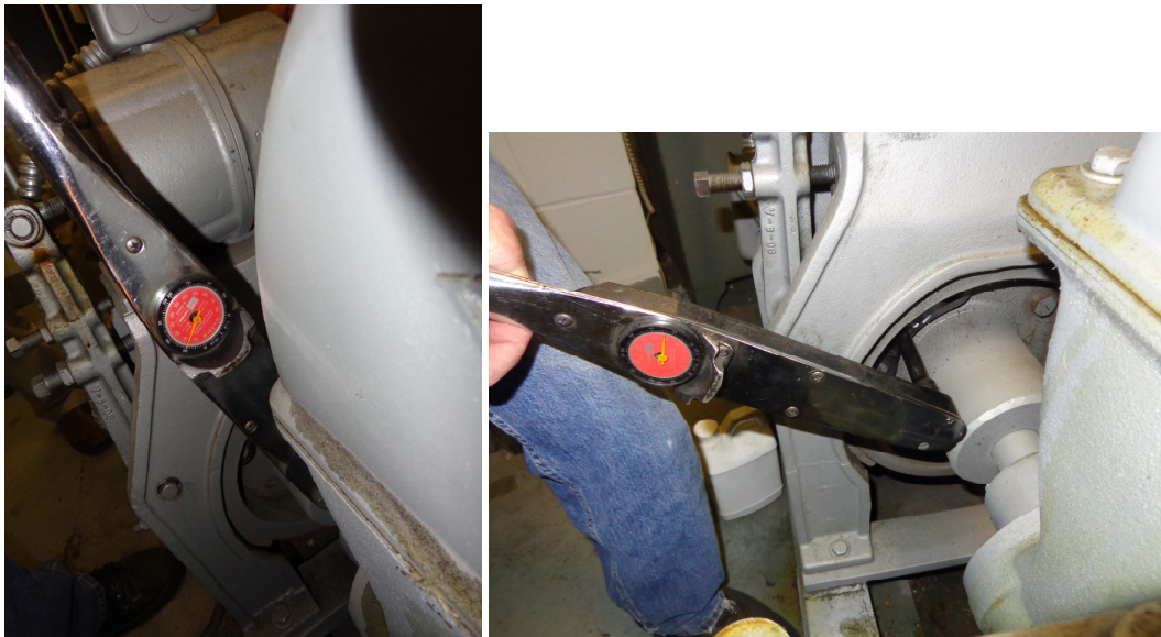
Figure 3 – Tool Placement: Drum Brake Testing, Disc Brake Similar, See Figure 1
