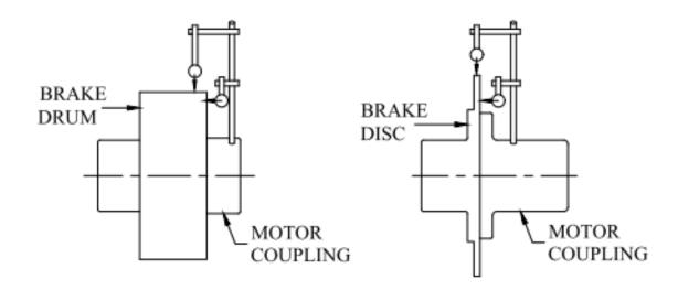
FIG. 1 - INDICATOR POSITIONING
