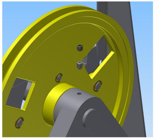
5. Remove two Set Screws (securing Main Shaft) from Governor Base.
