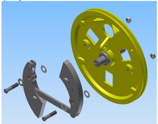
8. Mark Front of Pawl (fly-weight) Assembly to help with later re-assembly. Remove 2 Jam Nuts from back of Sheave/Shaft Assembly and remove (unscrew) Pawl Pivot Bolts. Again note number and location of washers on Pivot Bolt and Pawl. Remove the Pawl Assembly as a Unit. Remove also Washers between Pawls and Sheave.
