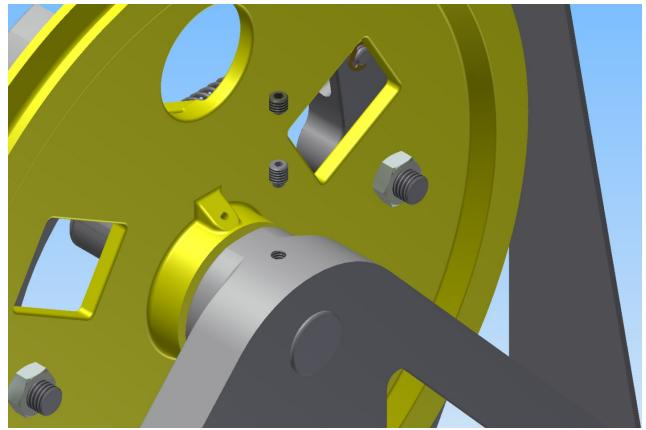
5. Remove two Set Screws (securing Main Shaft) from Governor Base.
