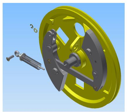
7. Remove E-clip (back of the Pawl (fly-weight)) from Tripping Spring Pin; remove Spring/Eyebolt Assembly, noting washer location.
