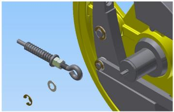
7. Remove E-clip from Tripping Spring Pin, remove Spring/Eyebolt Assembly, noting washer location.
