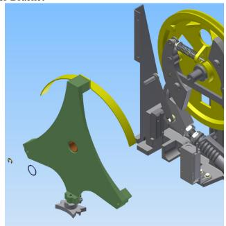
4. Remove E-clip from Link Pin, and Shaft Retaining Ring from Main Shaft and slip Yoke Assembly off Main Shaft. Slip Governor Rope off Sheave and secure it out of the way.
