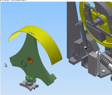
4. Remove E-clip from Link Pin, and Shaft Retaining Ring from Main Shaft and slip Yoke Assembly off Main Shaft. Slip Governor Rope off Sheave and secure it out of the way.
