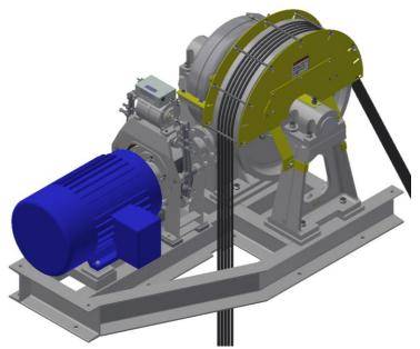
• Confirm all Hardware is tight. All Hardware is Grade 5 and should be tightened to Grade 5 Specifications.
