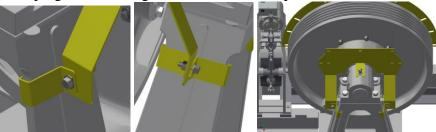
• Install Side Plate Assembly to the Side Plate Bracket. Tighten all clamping bolts, and the jam nut securely making sure the entire assembly remains square with the Traction Wheel.
