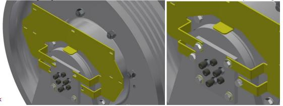
• For 63 and 74 Series Machines, securely bolt the Side Plate Assembly to the Side Plate Bracket as shown.
