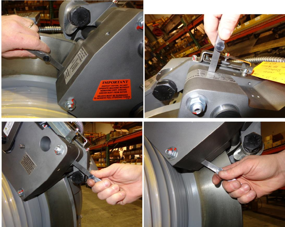
Figure 26: Air Gap readings 4 places around brake.
