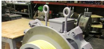
Figure 10: 2 lifting eye bolts installed (example)
