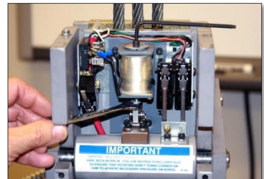
Figure 6: Brass Nut & Allen Screw Location
