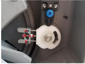
2. Rotate the over-speaed switch trigger to its normal (horizontal) operating
