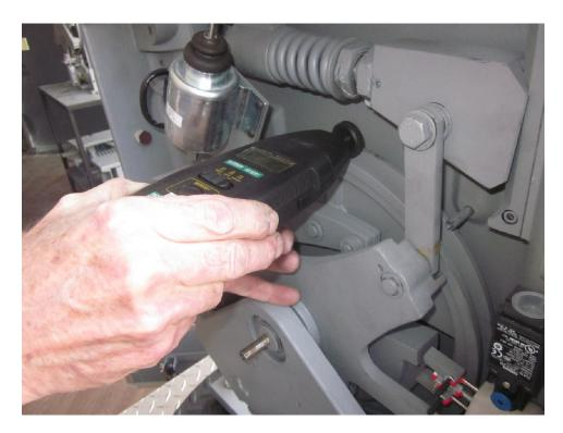
Figure 24 - Tachometer Placement Outside of Rim
