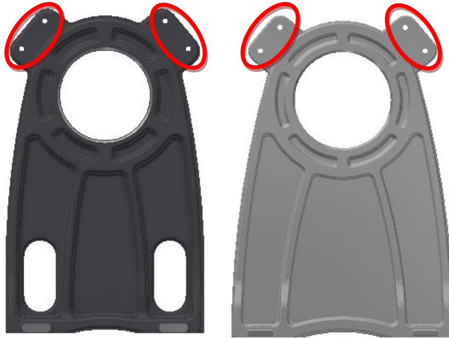
Figure 4-8: Mounting Holes on GT11 (left) and GT31 (right) Outboard Stands
